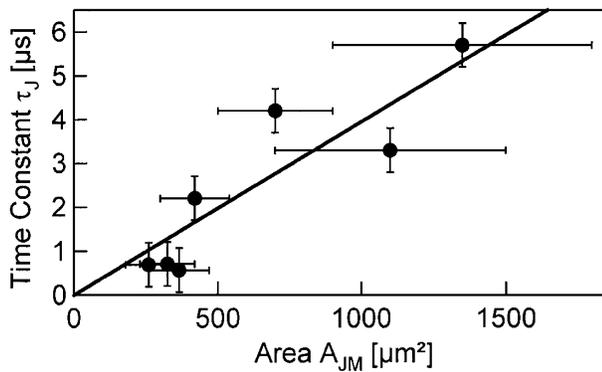
FIG. 4. Time constants  $\tau_J$  of optical transients near the center of adhesion of HEK293 cells versus the area  $A_{JM}$  of adhesion. The regression line has a slope of  $\tau_J/A_{JM} = 4.0 \text{ ns}/\mu\text{m}^2$ .
